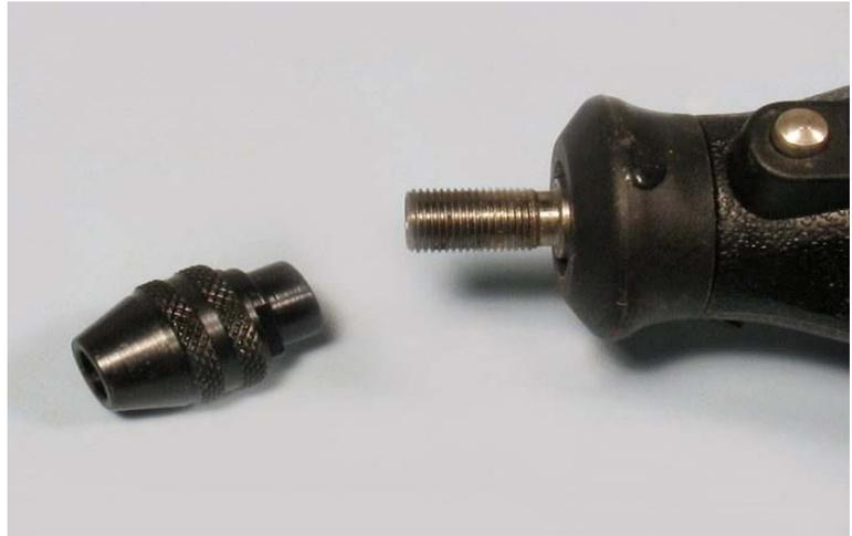
Many of us have a Dremel motor tool to use at home or when out to a class or workshop. The one thing that makes this tool much more productive is the addition of one inexpensive option, an adjustable chuck.
