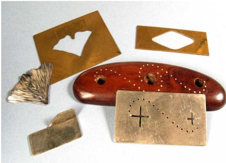
**Whenever I have to make more than 2-3 exact copies of a sheet metal component, I think of making a template. Templates let me easily draw the shape of an item to cut out.**
